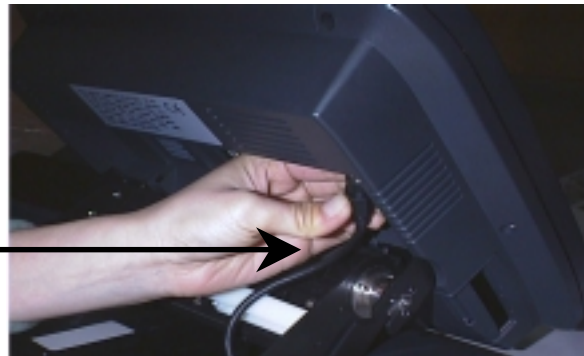
Figure 12: DC POWER INTERFACE
